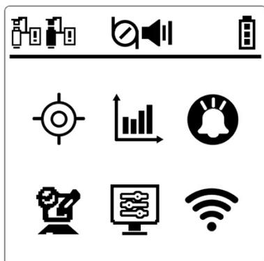
Press both the Up and Down keys simultaneously on the main screen to open the configuration menu on the left. The selected icon will be highlighted with a border. Use the Up or Down keys to navigate to the desired option, then press the Enter key to select it. The settings are available in the following order: Calibration → Measurement → Alarm → Log → Monitor → Wireless Settings.
