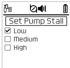
The pump blockage level can be set to High/Medium/Low. The default setting is **Low**.
