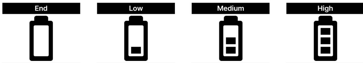
To charge the device, connect the provided charging adapter to the device, then plug it into an AC outlet. The device will display a rotating icon to indicate that it is charging until the battery is fully charged. Once the charger is removed, the battery icon will show the current battery status.
